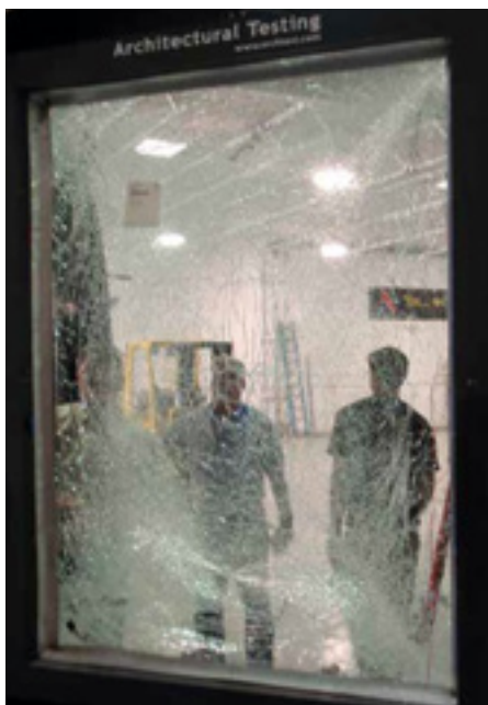
• A laminated glass panel is inspected after shock tube blast testing (above), to assess glass fragmentation.
